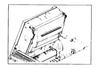
2. While holding down the green master unit release lever, slide out the master unit (lift the green ledge as shown in the diagram).
